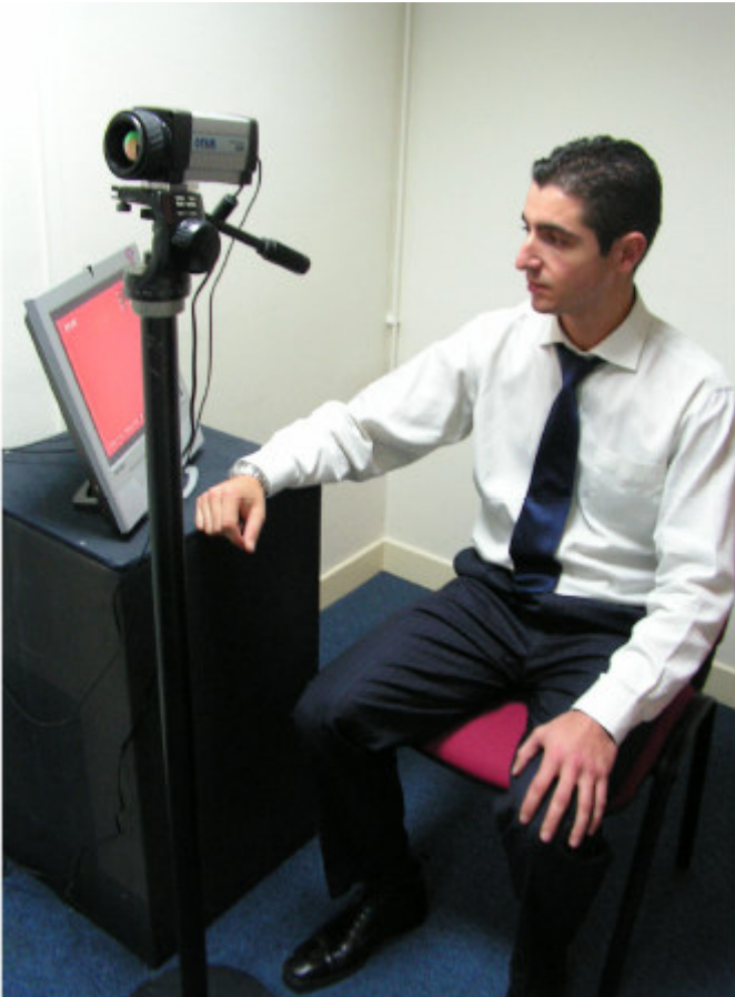
Installation THV A20M - SARS example: a video screen is necessary if you want to see thermal images coming from the camera
